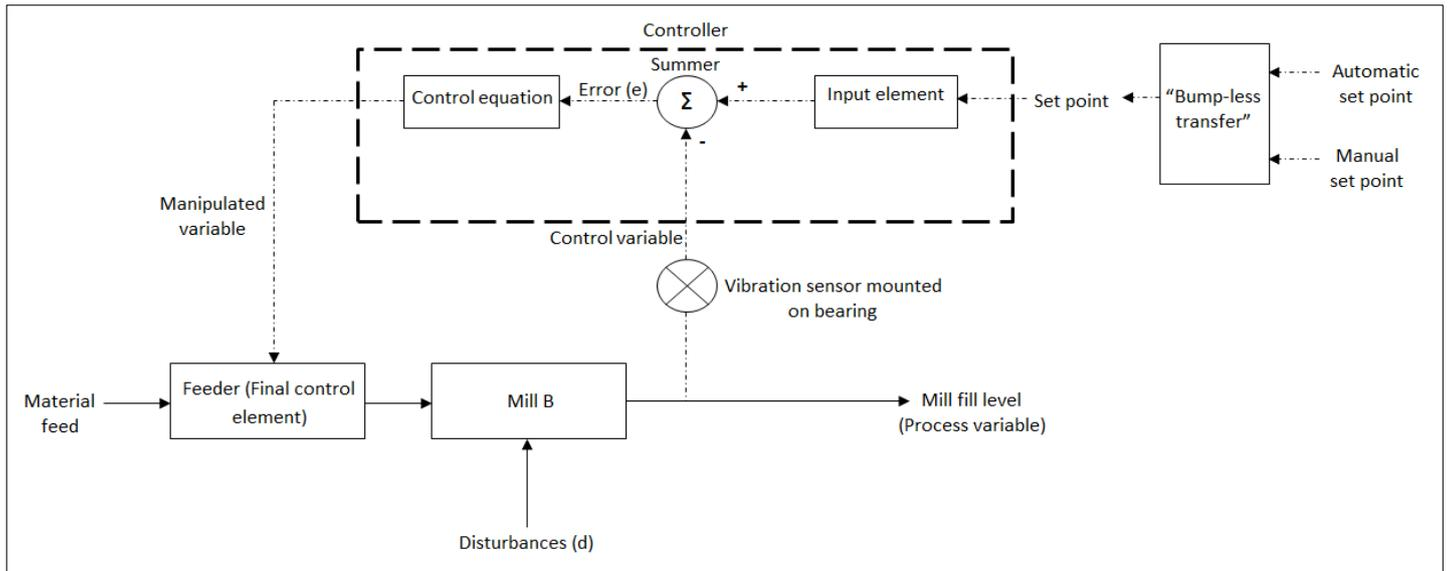
Figure 4-1: MillScan level controller block diagram.
