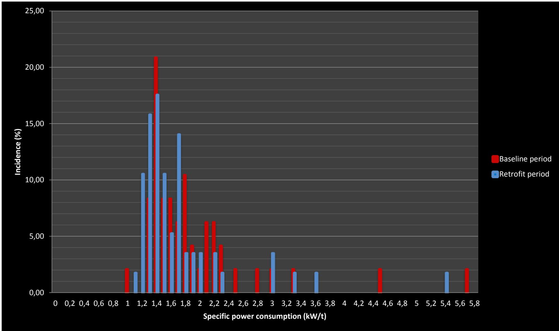
Figure 9-1: Histogram of the specific power consumption data from mill B.
