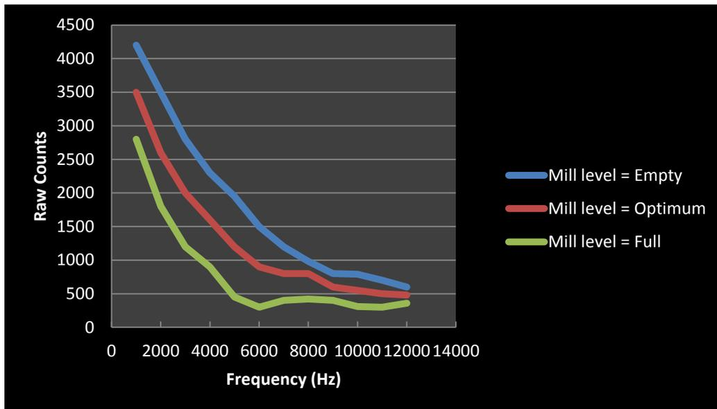
Figure 7-2: Vibration snapshot of various mill fill levels.
