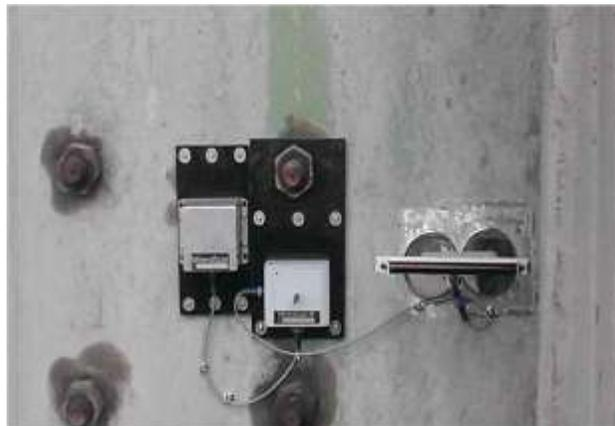
Figure 2 - Shell Mounted Components: Battery, Transmitter, T-Sync (left to right)
