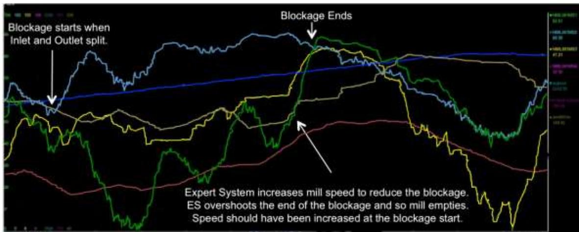
Figure 7 - Expert System Bearing Pressure Control - Blockage - 1 Hour Duration
