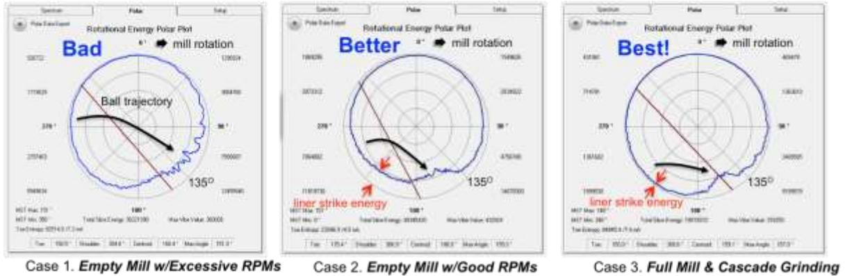
Figure 4 - Mill Conditions: Too Fast, Too Empty, Full Mill (left to right)
