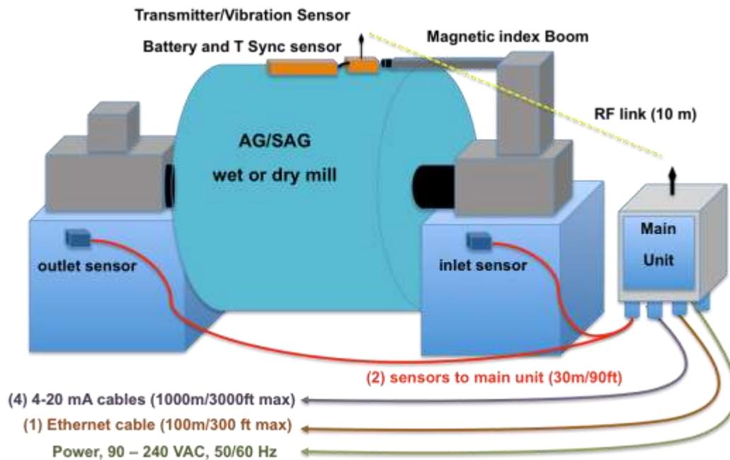
Figure 1 - Vibration System Components
