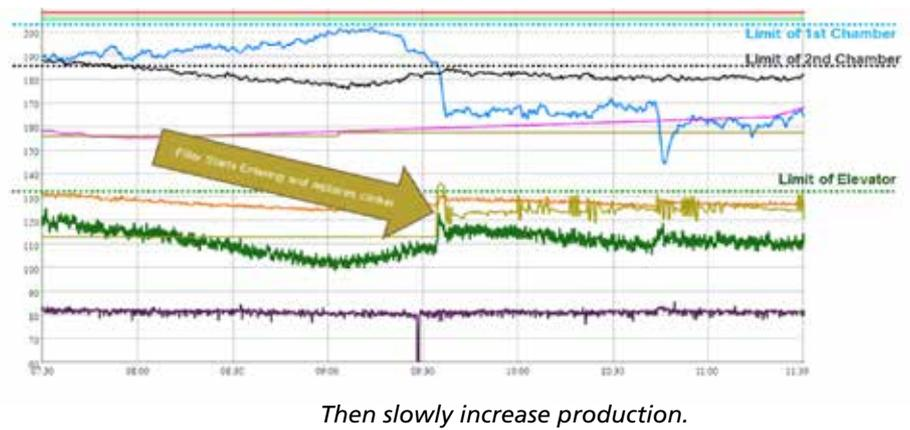
Figure 4. Injection of filler at the elevator.
