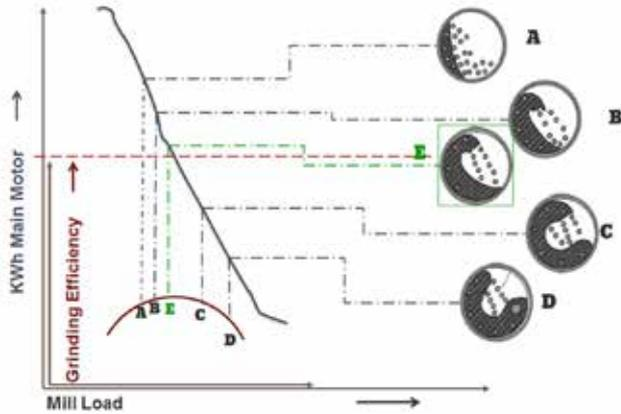
Figure 2. Mill Motor Power (KWh) vs. Mill Material Loading.
