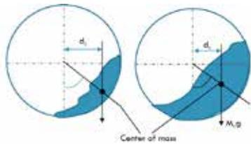
Figure 1. Center of Mass ( $M_c$ ) vs. Mill Load.
