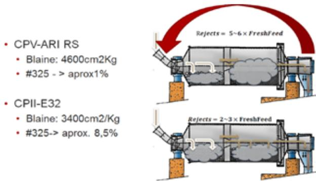
Figure 3. Material flow differences according to cement type.
